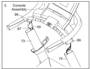
Finger tighten three Handrail Bolts (64) with three Upright Star Washers (90) into the Right Upright (74). Next, finger tighten three Handrail Bolts with three Upright Star Washers (not shown) into the Left Upright (73). Then, firmly tighten the six Handrail Bolts.
